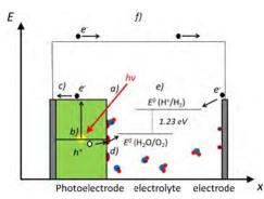
**Figure 1**. Scheme illustrating the main phenomena involved in photoelectrochemical water splitting, where a photoanode is immersed in an aqueous electrolyte. a) light-matter interaction, b) electron-hole pair generation, c) charge separation and transport, d) catalysis and e) the water-splitting reaction, and f) photocurrent associated with the photoelectrochemical (PEC) water splitting.
